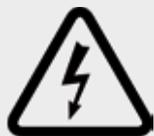
This symbol indicates the possible electric shock hazard associated with uninsulated live components in the interior of the unit.
